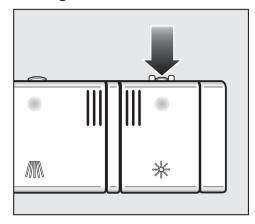
■ Press the button on top of the rinse aid reservoir in the direction of the arrow. The cover will pop open.
